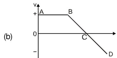
**Sol.** (a) **During interval AB:** velocity is +ve so the particle is moving in +ve direction, but it is slowing down
