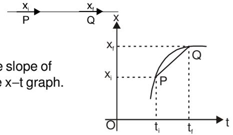
This expression suggests that the average velocity is equal to the slope of the line (chord) joining the points corresponding to P and Q on the  $x-t$  graph.
